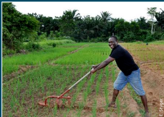
Pascal Gbenou, demonstrating a cono weeder on his field in Kakintchoué, Benin, April 2013
