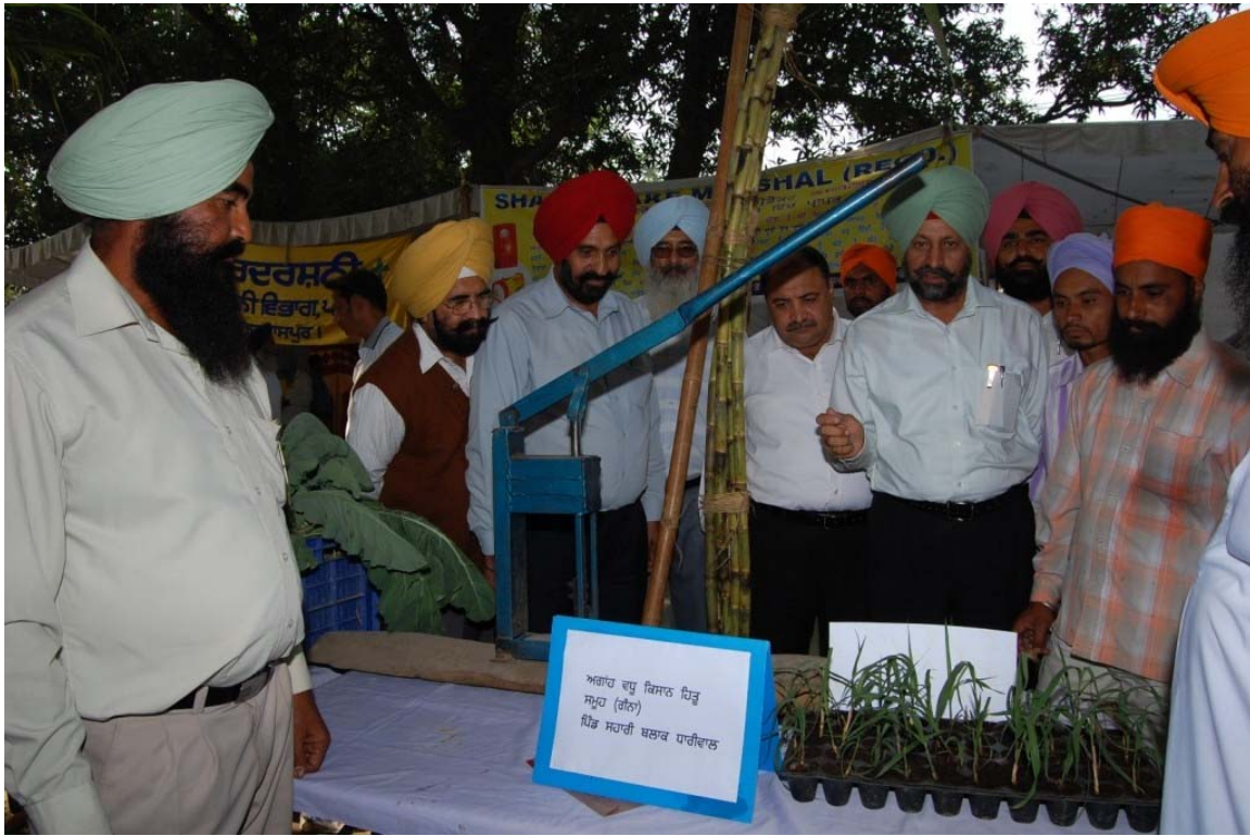
Figure 1: Bud chipper implement for cutting out buds from sugar cane
