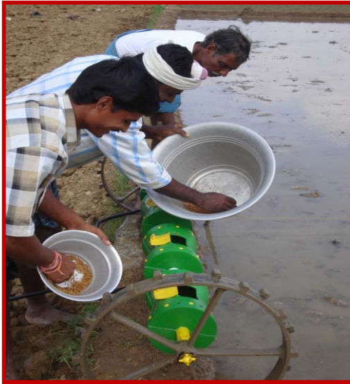
Filling of pre-germinated paddy seed into the drums
