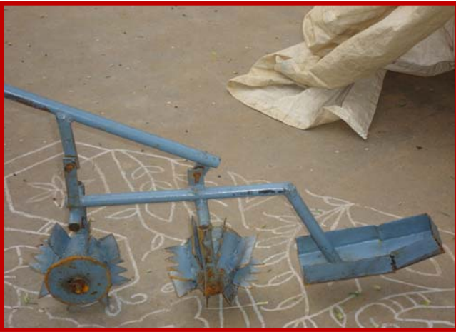
Modified conoweeder with two wheels, each of 12.5 cm width, to fit into 20 cm row spacing of direct-seeded rice
