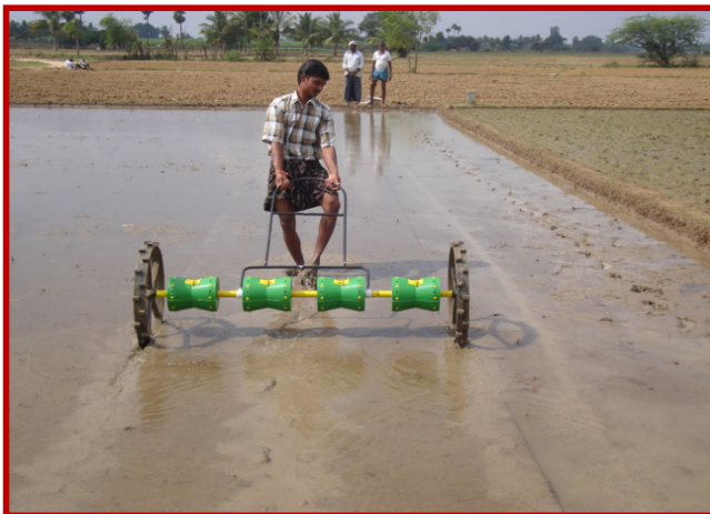
Pulling the drum-seeder in the puddled field without any standing water
