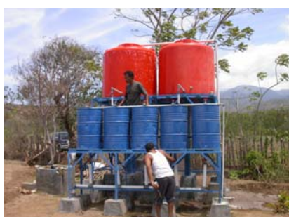
Irrigation supply measuring tank
