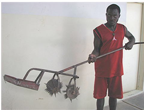
Above left: A “Cono” rotary hoe push-weeder developed at the WARDA Sabel Station for use in SRI fields. Right: The weeder in use in an SRI field in the cuvette of Nianga, Podor.
