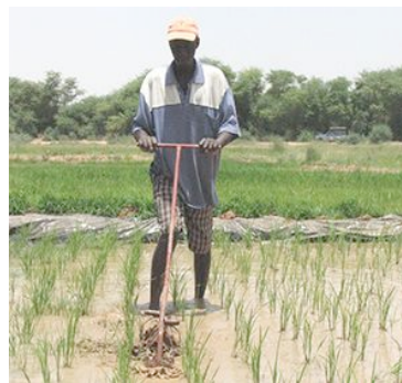
Above left: A “Cono” rotary hoe push-weeder developed at the WARDA Sabel Station for use in SRI fields. Right: The weeder in use in an SRI field in the cuvette of Nianga, Podor.
